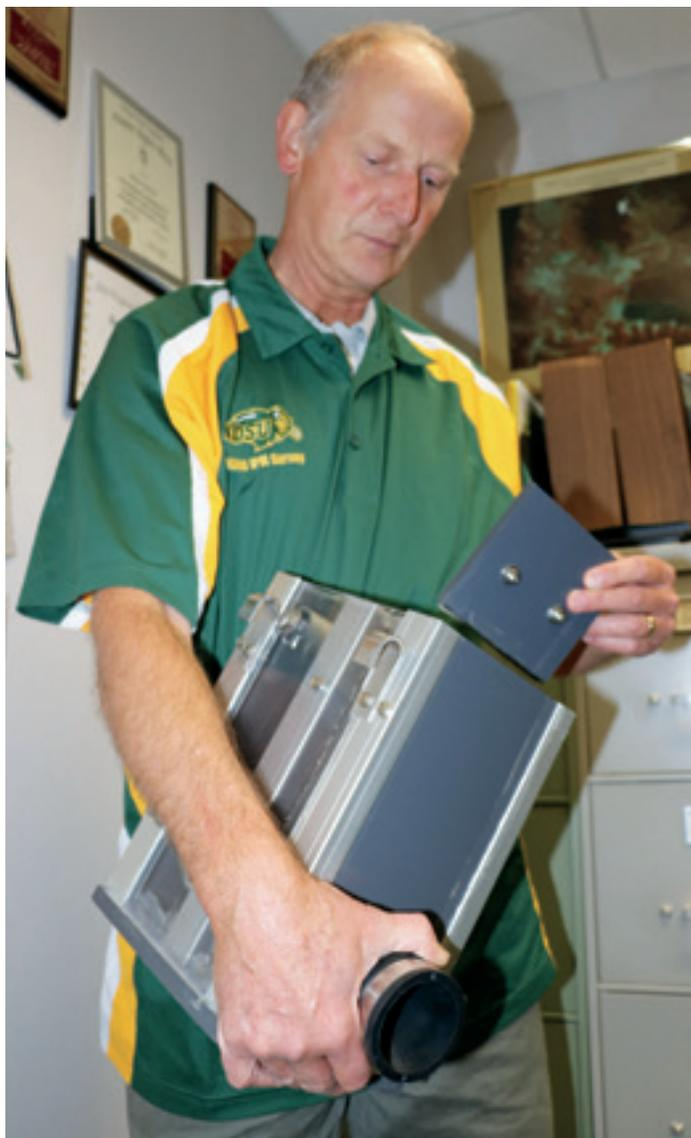
NDSU researcher Dr. Hans Kandel holds a tabletop control box. When connected to subsurface tile drainage, control boxes can help farmers manage the water table in their fields.
