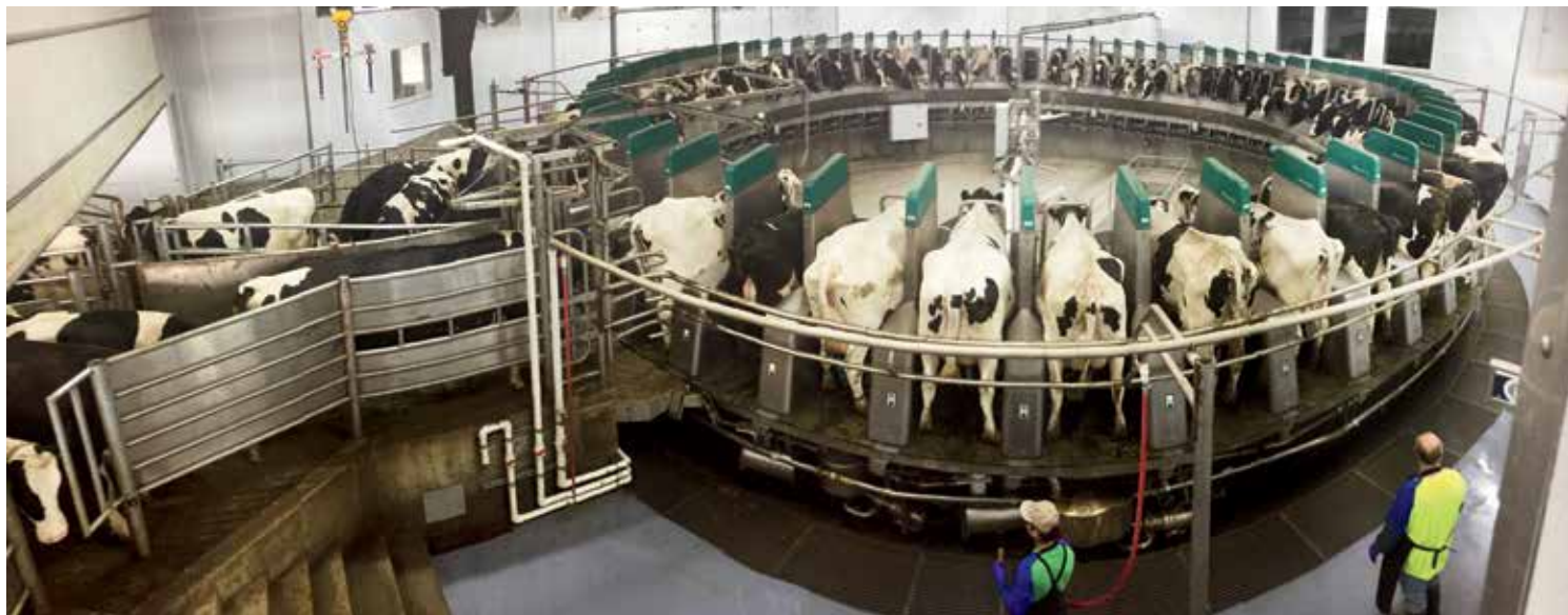
A 60-cow platform is about 70 feet in diameter. Cows go onto the platform that is provided with 60 robot milkers. They are milked in 5 to 7 minutes, before exiting after a 9-minute rotation, or one every 10 seconds.
