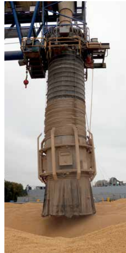
Soybeans are conveyed from storage bins and loaded onto cargo ships through massive spouts.
