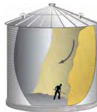
Try to break up a vertical wall of grain from the top of the bin, not the bottom, because the grain can collapse and bury you.
