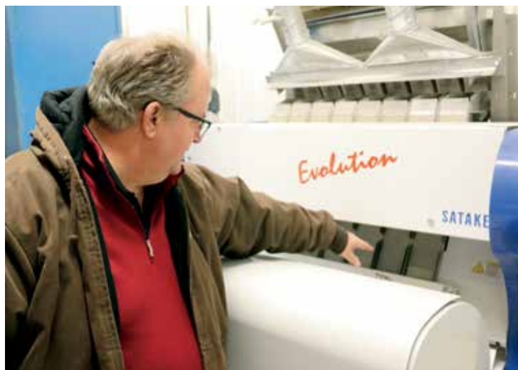
Carl Peterson highlights equipment that can evaluate 50,000 soybean seeds per second.
